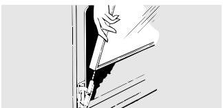
Lift the door straight up and off the hinges.
